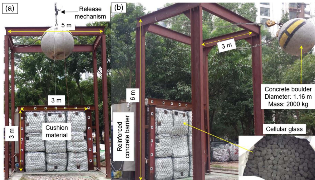
Fig. 2. Impact test setup: (a) front view; and (b) oblique view.
